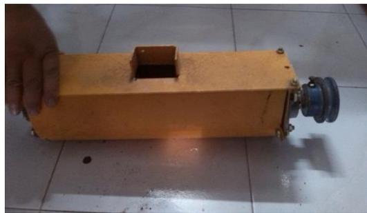
Gambar 2. *Housing Screw Conveyor*
